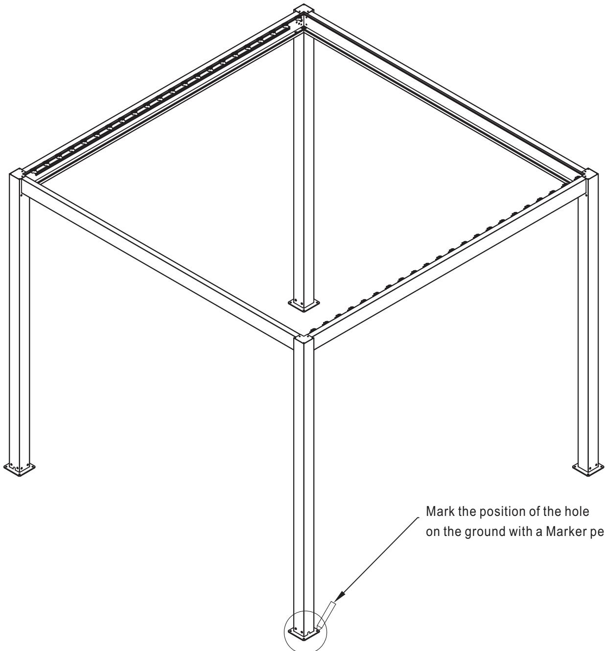
Tool used: marker pen(to be provided by the installation worker)
