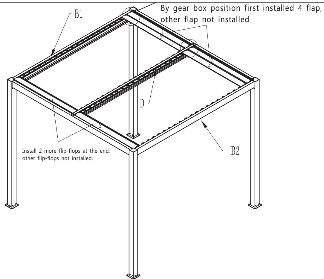
13.Tighten and fix the screw k 3 in step 11, and then fasten the remaining flap in turn.
