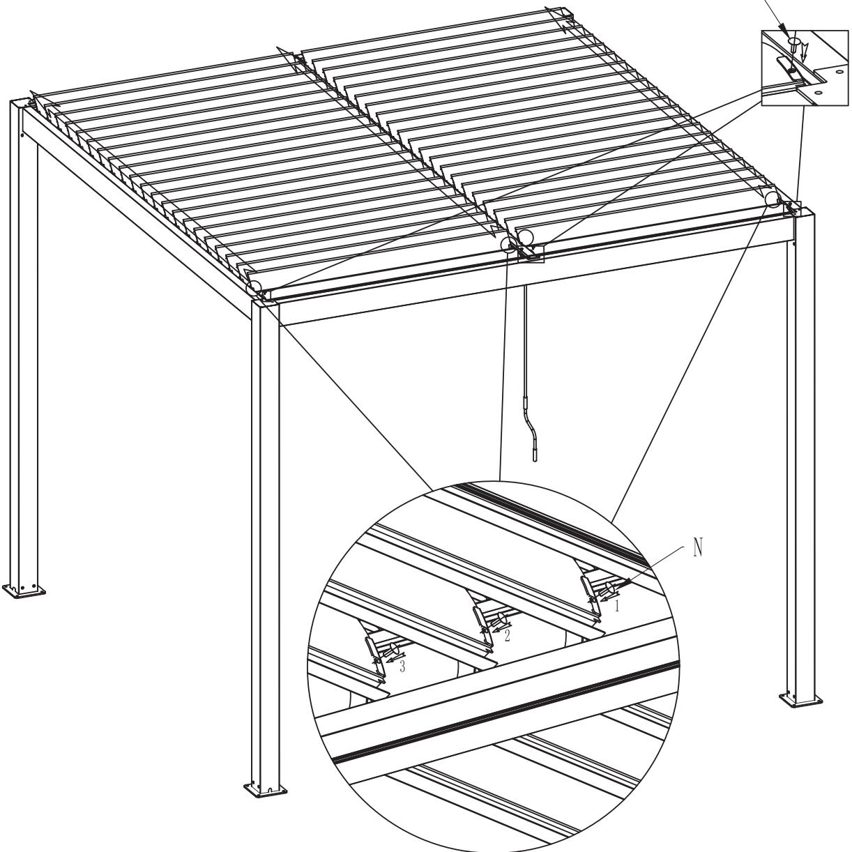
Step 5.Open the flap in half and insert the plastic plug n into the plug mounting holes at both ends of the flap as shown in the drawing in the upper circle.
