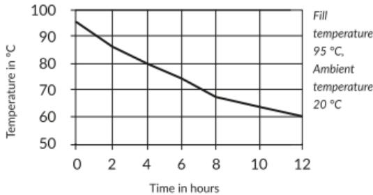
Temperature profile for cold drinks in the 0.75 l Thermocafé insulating drinking flask
